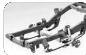
DURABLE RIGID FRONT LEAF SPRING SUSPENSION
